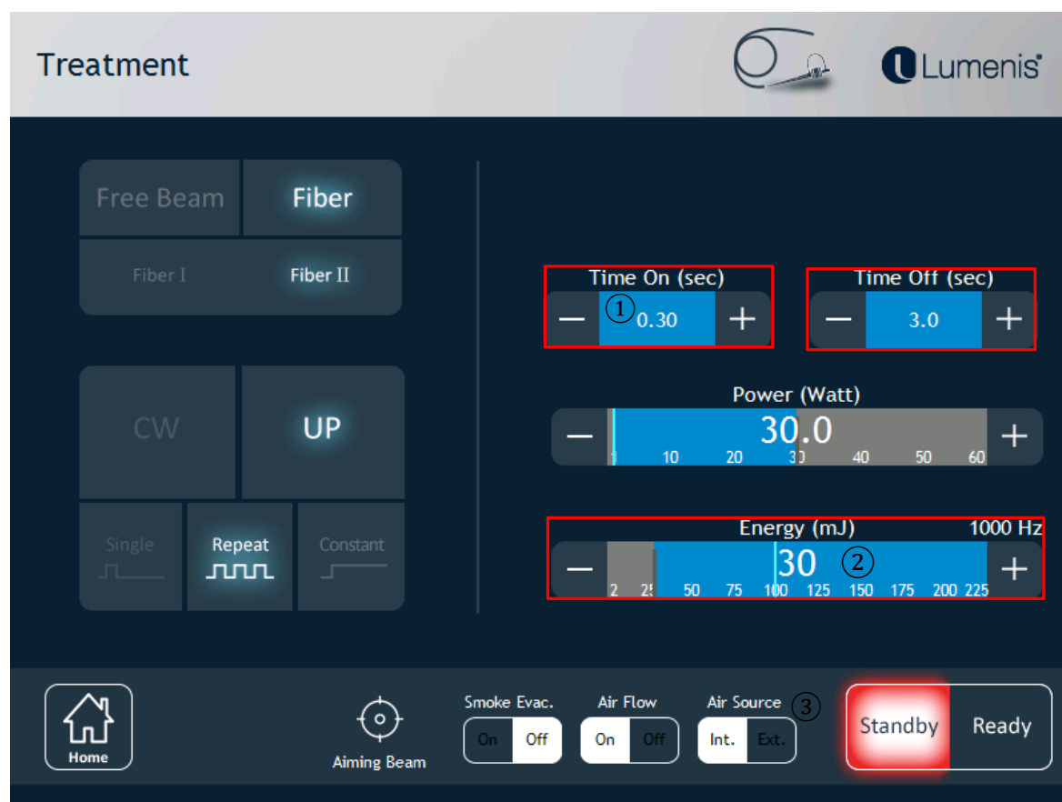
Figure 5-8: Treatment Screen – Fiber UP Repeat Mode
