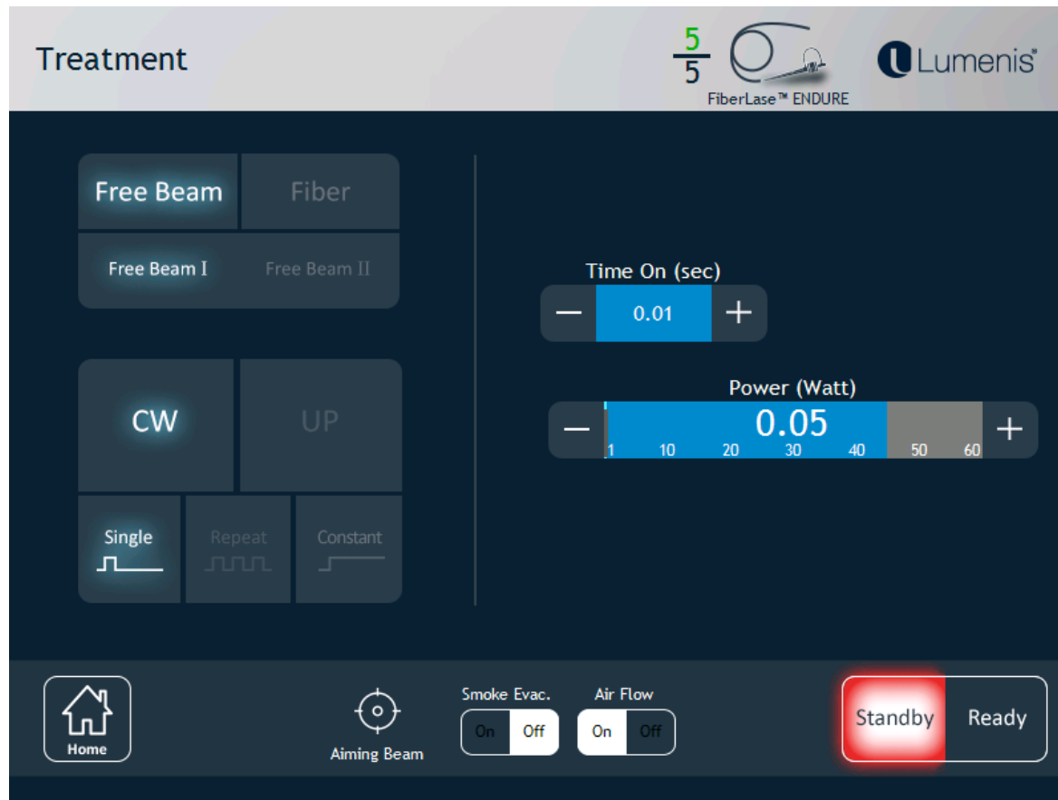
Figure 5-6: Elements of a Treatment Screen
