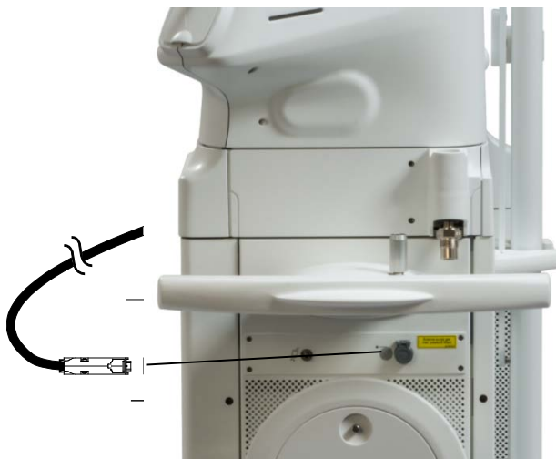
Figure 4-10: Connecting the Scanner Communication Cable to the Laser Console
