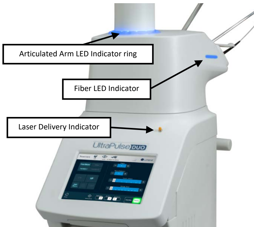
Figure 2-2: CO 2 Laser Output Port Indicators
