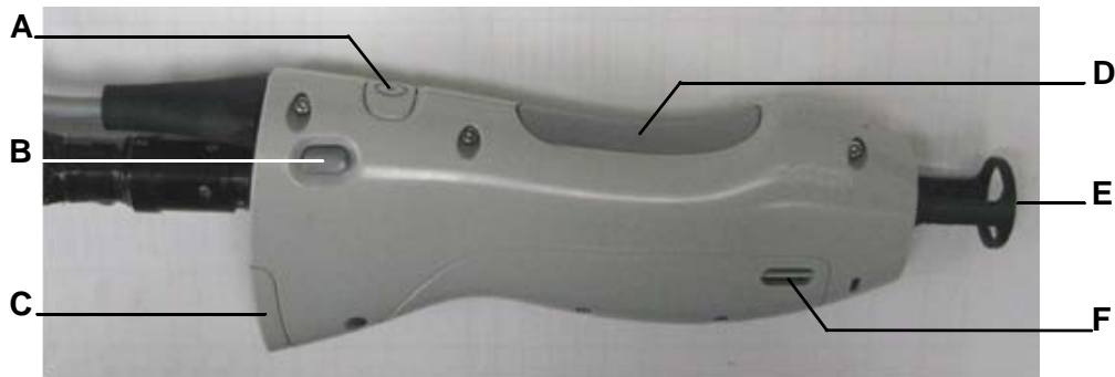
Figure 2-3 Specialty DCD Handpiece Components
