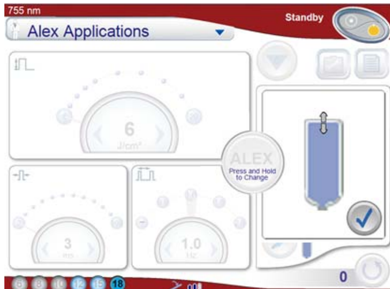
Figure 3-7 Cryogen Level Indicator: Estimated Full Canister
