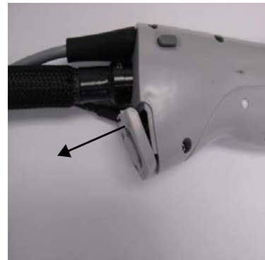
Figure D-2 Removing the DCD Handpiece Fan Filter Cover
