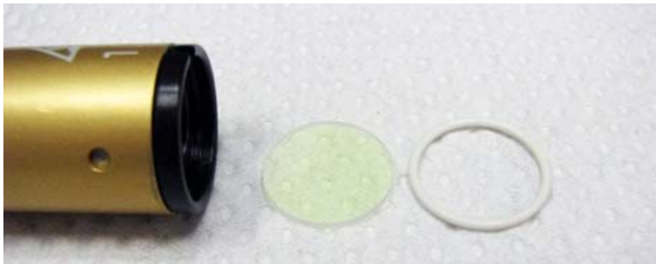
Figure B-24 O-ring and Window Removed
