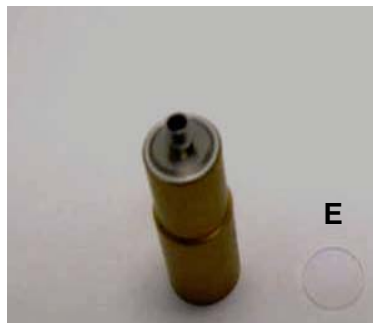
Figure B-18 Removing the Window from the Slider Attachment
