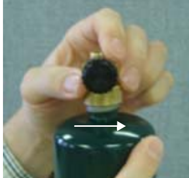
Figure D-13 Putting the Venting Valve on the Canister
