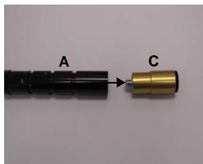
Figure B-16 Removing the Slider Attachment from the Slider
