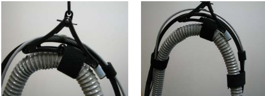
Figure 2-21 Attaching the Cooling Hose to the GentleMax Pro Cradle
