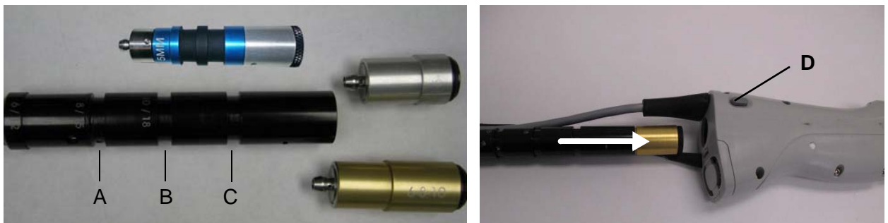
Figure 4-2 Inserting the Fiber Cable into the Handpiece (DCD shown; same for ACC)
