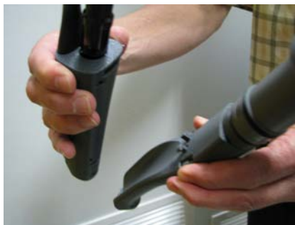
Figure 2-8 ACC Handpiece Removed from the ACC Air Clip
