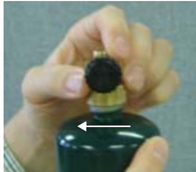
Figure D-11 Putting the Venting Valve on the Canister
