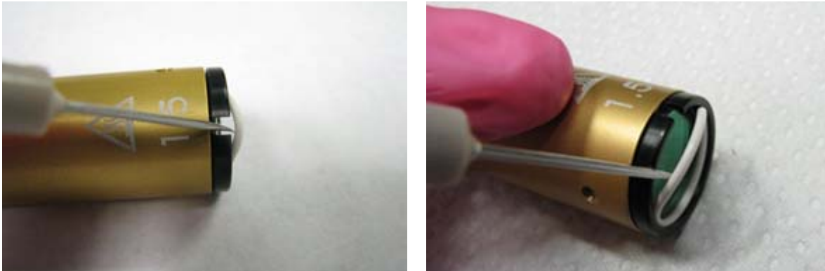
Figure B-23 Removing the O-ring
