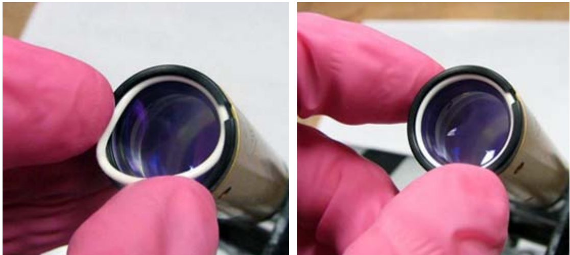
Figure B-26 Installing the O-ring
