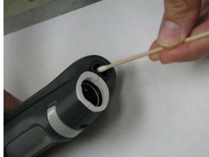
Figure B-10 Cleaning the ACC Air Cooling Aperture
