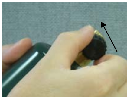
Figure D-12 Purging the Cryogen Canister
