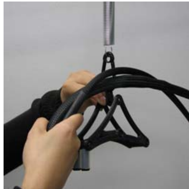
Figure 2-17 Inserting Delivery System Cables in the Cradle
