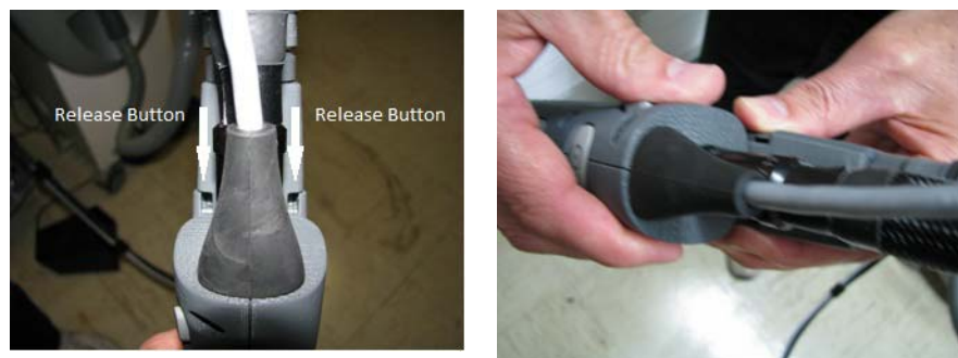
Figure 2-7 Releasing the ACC Air Clip
