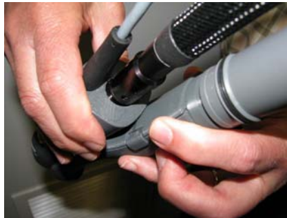
Figure 2-6 Locking the ACC Air Clip
