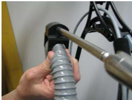
Figure 2-20 Attaching the Cooling Hose to the Cooling Device Pole
