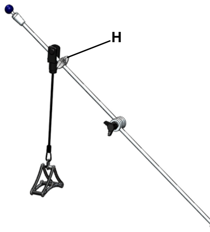
Figure 2-15 Adjusting the Clip to Limit Sliding
