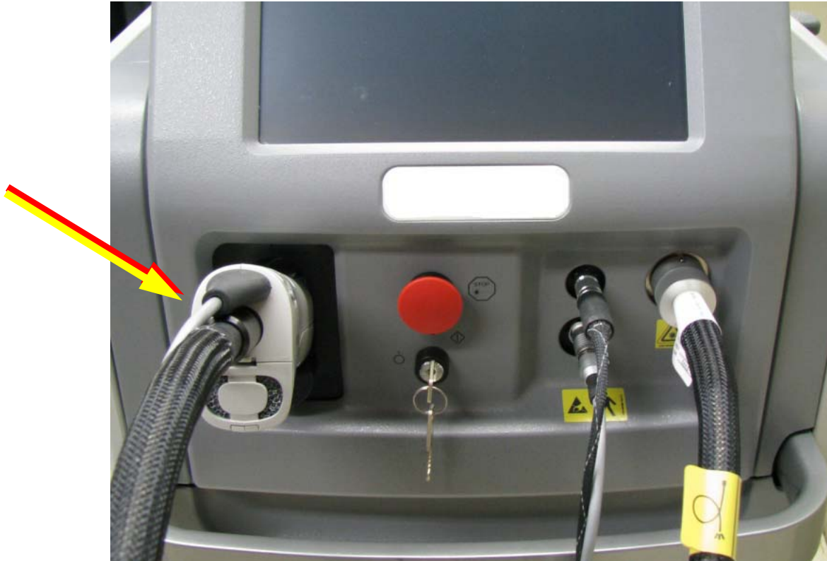
Figure 4-3 ACC or DCD Handpiece Fully Inserted Into Calport
