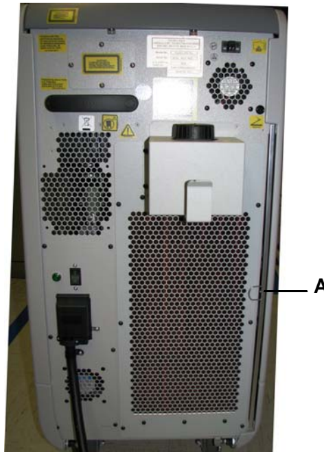
Figure B-1 Location of the Air Filter (Rear Panel View)
