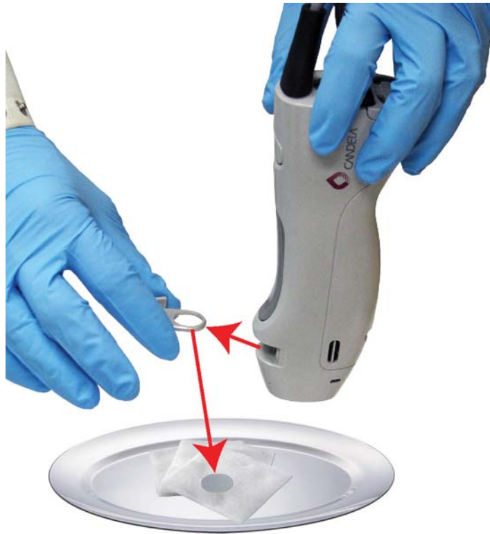
Figure B-3 Removing the Standard Handpiece Window Holder
