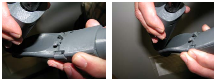
Figure 2-5 Attaching the ACC Air Clip
