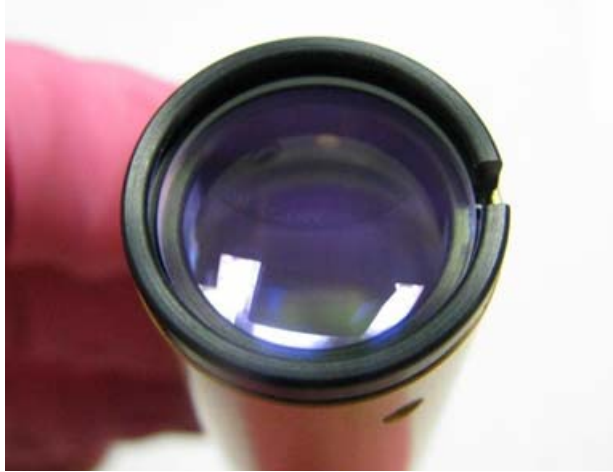
Figure B-25 Window Installed in Slider Attachment
